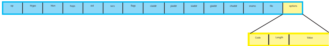
Figure 11-1. DHCP Packet Format
